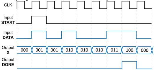
Derive the state transition diagram for this circuit.
